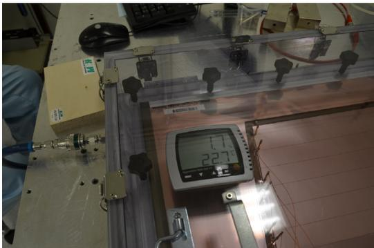
(k) One of three hygrometers in the test box to verify the required measurement conditions
