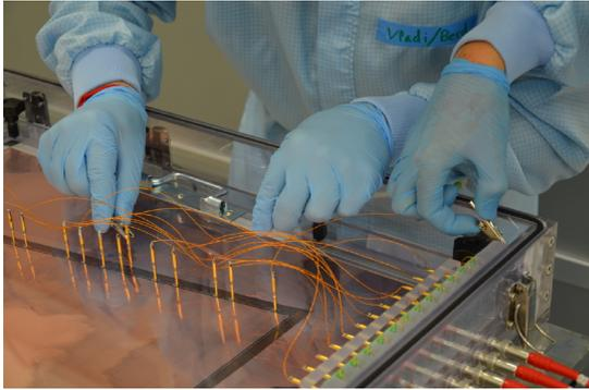
(i) Establishing connection from the *ground pin* to the test box
