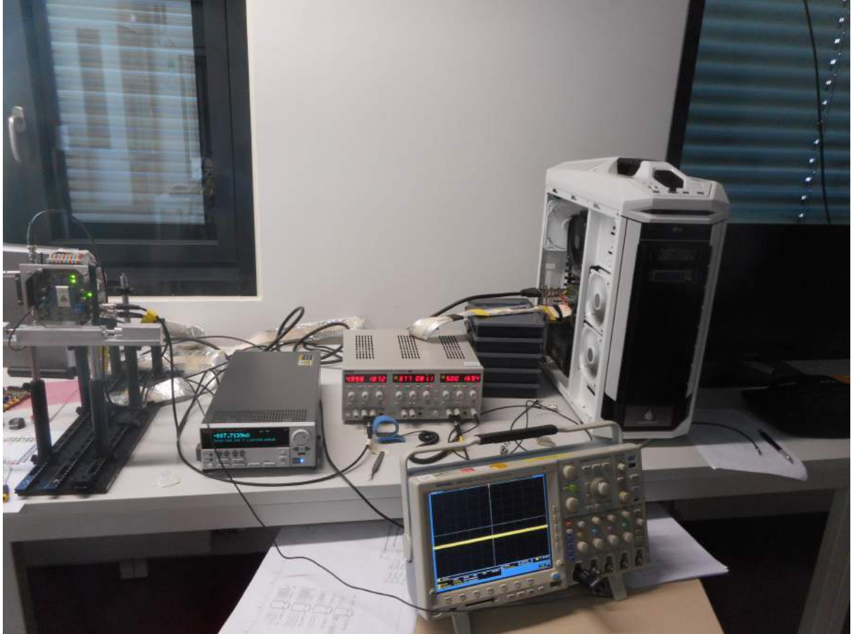
Figure 8.2: Single setup. From left to right: MuPix PCB in a custom metal frame with the iron source covering the chip, the power supply for the HV [29], the power supply for the low voltage [30] to power the chip and PCB, oscilloscope and the computer housing the FPGA.
