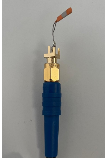
Figure 19: Capacitor soldered onto a SMA-connector for the validation measurements.
