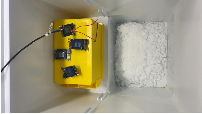
Figure 24: Cooling Setup with dry ice used in this thesis.
