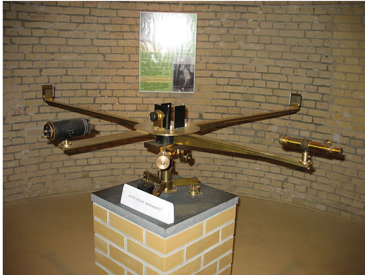
replica of the Michelson-Morley experiment in Potsdam (source: Wikimedia Foundation)
