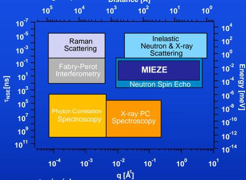
To cover high q ranges and large interaction times a fast detector is needed for the MIEZE technique
