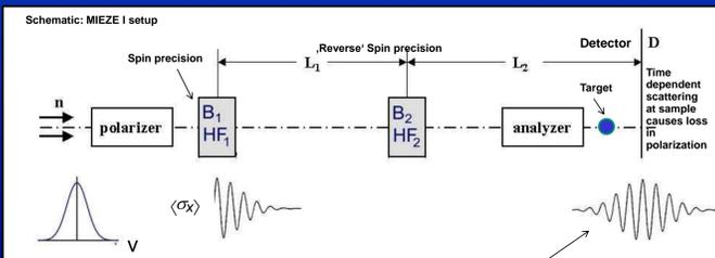
Example: Frequency 654kHz, λ<sub>n</sub> = 5 Å, v = 800m/s, Spin-Wavelength of signal: 1.2 nm
