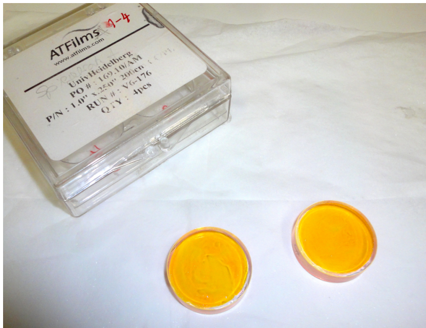
Figure 5.3: Picture of two highly reflective cavity mirrors. The mirrors in this image are still coated with a polymer to prevent dust and other particles from reaching the reflective surface.
