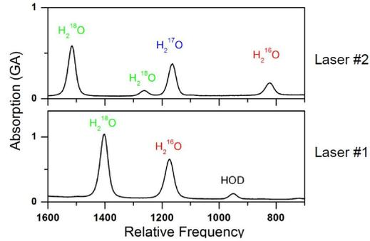
Figure 3.2: Absorption spectra of the two lasers from (BAER 2013).
