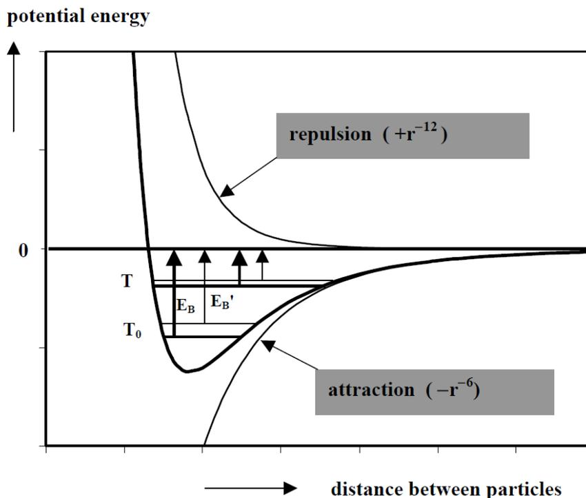
Figure 2.1: Schematic representation of the potential energy distribution of a diatomic molecule. The resulting shape of the energy well is caused by the counteracting repulsive and attractive forces between the two particles. The arrows indicate the binding energies for the considered heavy/light isotopic molecule. Figure taken from MOOK (2000).
