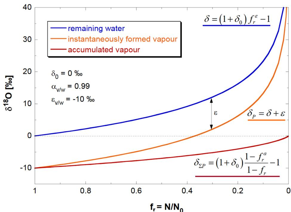
Figure 2.3: Changes in isotopic composition during Rayleigh fractionation process in a closed system. The reservoir has an initial isotope ratio  $\delta^{18}\text{O}$ . The fractionation factor is  $\alpha = 0.99$ .
