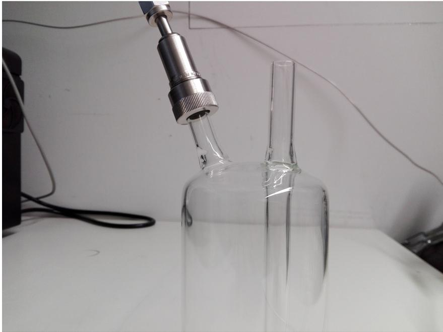
Figure 5.3: Setup for experiment 5.2: end of the instrument line connected to the cooling trap. The drop is inserted through the vertical opening.
