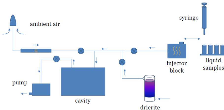
Figure 3.4: Principle of the two mode analyzer. Measurements of ambient air (left part of the set-up) and of liquid samples (right part of the set-up) are possible.
