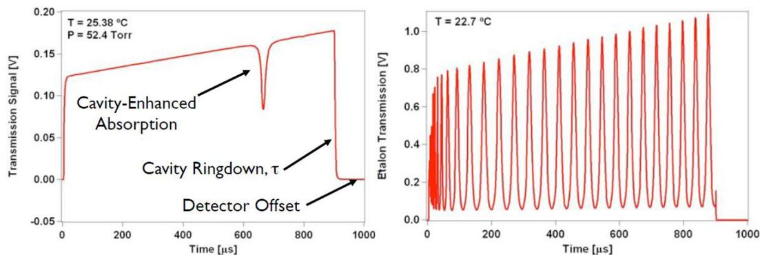
Figure 3.3: Transmission signal of the cavity and transmission through the etalon, dependent on time (BAER 2010).
