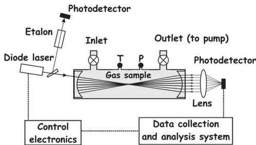
Figure 3.1: Schematic of instrument setup for OA-ICOS from (BAER ET AL. 2002).
