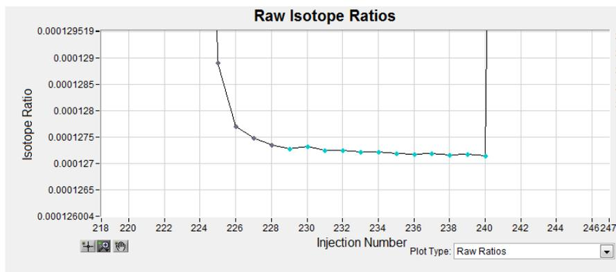
Figure 6.2: Injections with high disparity in isotopic values can cause memory effects on the raw ratios. When measured twice all injections except for the last four must be discarded manually.
