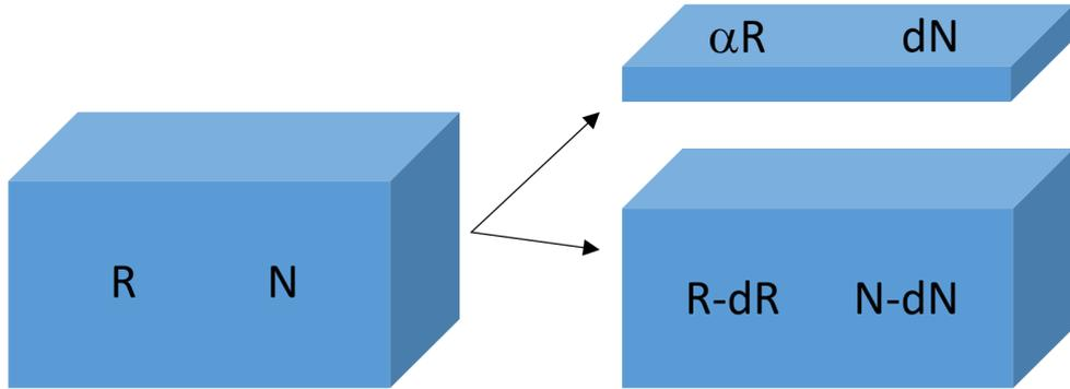
Figure 2.2: Schematic view of a Rayleigh fractionation process considering an initial reservoir with  $N$  molecules and isotopic ratio  $R$ . During evaporation, an infinitesimal  $dN$  is removed and its isotopic signature is altered by the fractionation factor  $\alpha$ .
