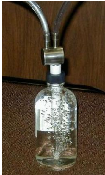
Figure 5.6: Glass frit, from Durridge [2001]
