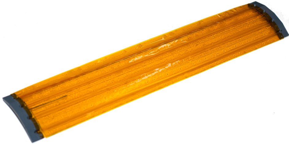
Figure 4.4: Prototype of Layer 3 module with 50 \mu\text{m} thick glass plates to simulate the flexibility of silicon. The shown, outdated prototype has only one V-fold.
