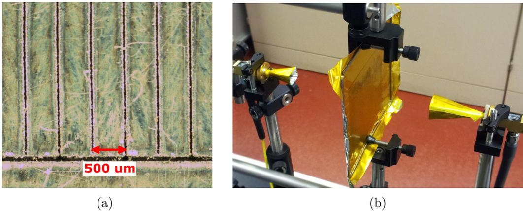
Figure 5.12: (a) Microscopic view of the polarising filter produced via laser ablation. (b) Setup mounted in the laboratory - back view of the polariser.
