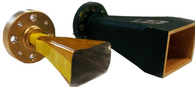
Figure 5.6: Aluminium Kapton horn antenna and brass standard gain horn
