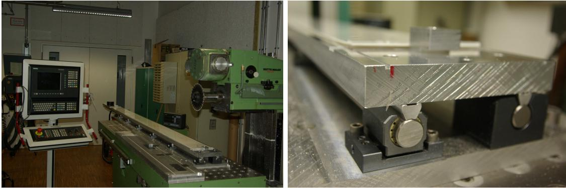
Figure 6.4: *Left*: Picture of the milling machine with the aluminium jig for the longitudinal cut. *Right*: Detailed view of the template with a rail system to extend the range of the machine to 2.5 m. [9]
