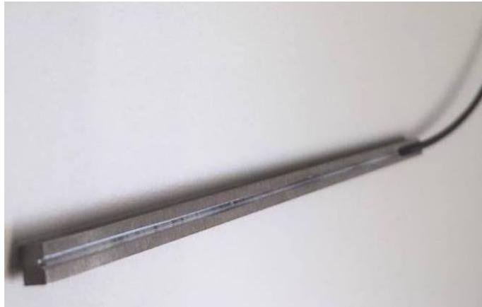
Figure 3.10: Picture of a lightbar with the optical fibre glued into an aluminium bar.
