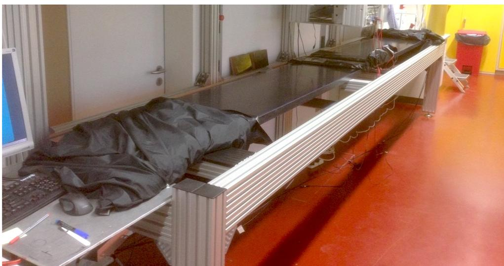
Figure 6.8: Full size fibre module measurement setup. Both ends are covered with black blankets. Two large scintillator paddle trigger are placed near the mirrors for each of the module sides.
