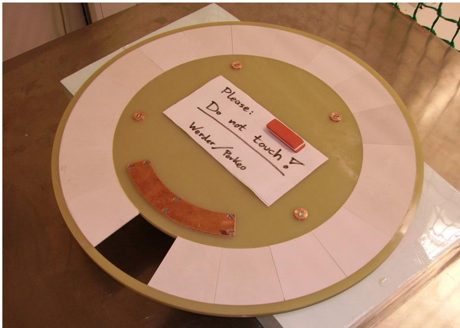
Figure 2.4: The finished chopper disc. One can see the  ${}^6\text{LiF}$  tiles used as the neutron absorber, the chopper opening angle of  $\alpha_C = 22.11^\circ$  and the balancing weights made of copper. The joints between the tiles feature a slight step which guarantees a maximum neutron transmission of  $8.8 \cdot 10^{-5}$ .
