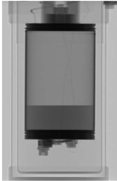
Figure 3.14: Neutron Radiography of experimental volume during condensation. Exposure time 30s, L/D=800 . The ^4\text{He} is clearly visible in the cell through the scattering cross section. At the bottom of the cell, the heater and the Lakeshore thermometer, both screwed
