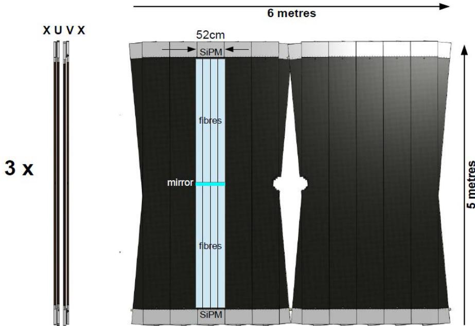
Figure 3.2: Schematic of the SciFi Tracker in  $yz$ - and  $xy$ -plane. One module is highlighted in blue and the segmentation of the eight fibre mats is indicated[8].
