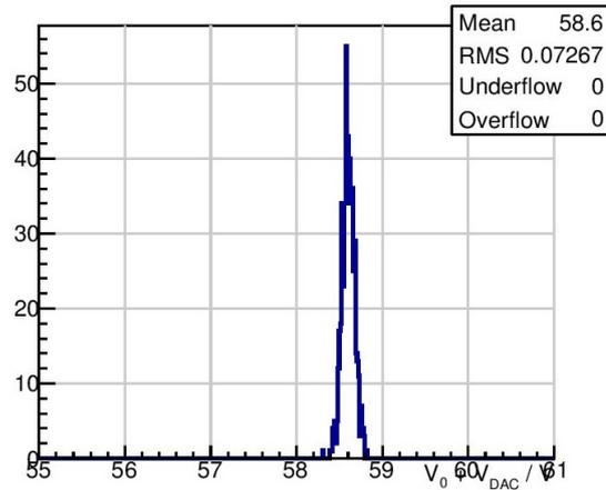
Figure 4.13: RMS for the breakdown voltage over all channels after gain calibration
