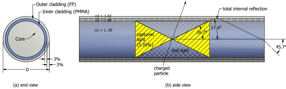
Figure 3.3: Schematic of the structure of a scintillating fibre from end view (a) and side view (b)
