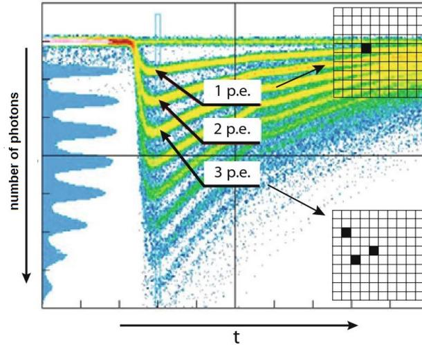
Figure 3.8: Pulses for different numbers of firing pixels. [12]
