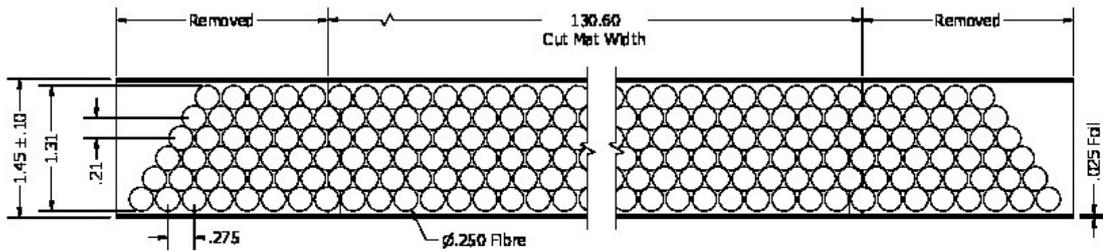
Figure 3.5: Schematic view of an uncut fibre mat with 6 layers. The sides will be removed so that the mat will have a width of 130.5 mm and a length of 2.5 m[2].
