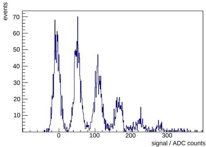
Figure 4.6: Spectrum of the light for one channel of the SiPM
