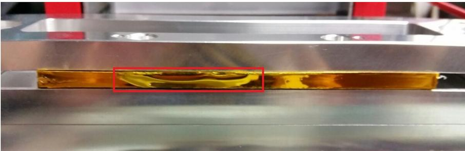
Figure 4.18: Mirror damage after the longitudinal cut of mat FIM00028
