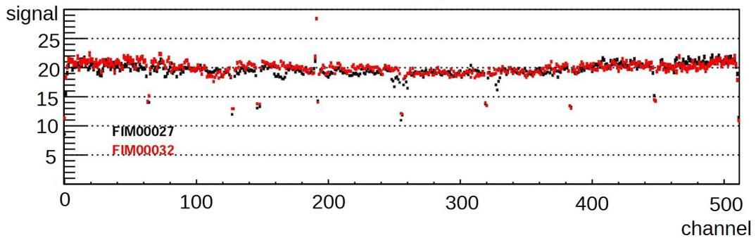
Figure 4.14: Measured light yield of the fibre mats FIM00027 and FIM00032. Their average is used as reference mat.
