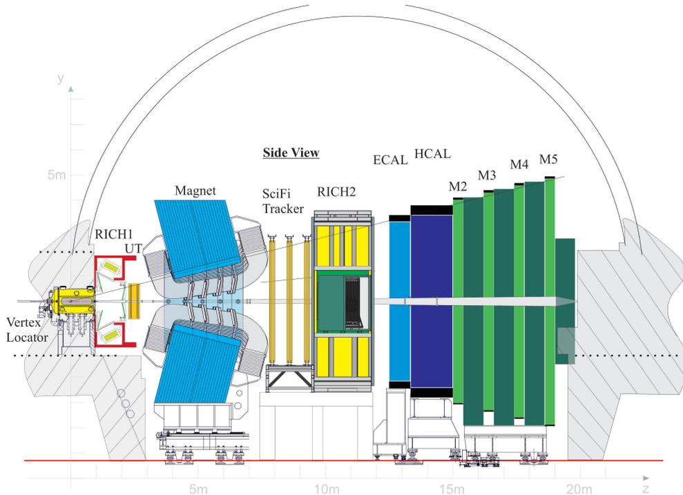
Figure 3.1: Schematic side view of the upgraded LHCb detector [1]
