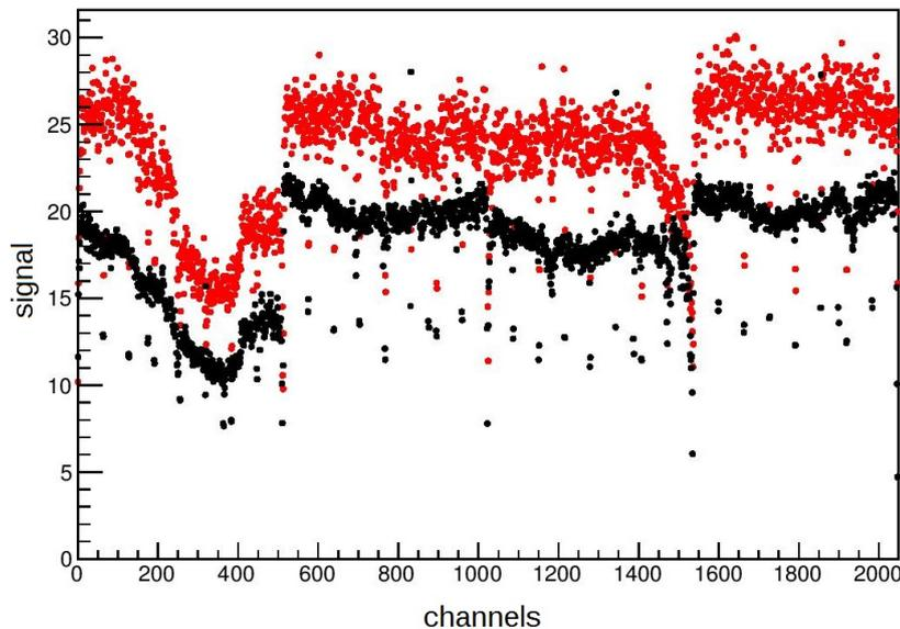
Figure 6.3: Measured light yield of the module in comparison to the light yield measured from the single mats with beta-source
