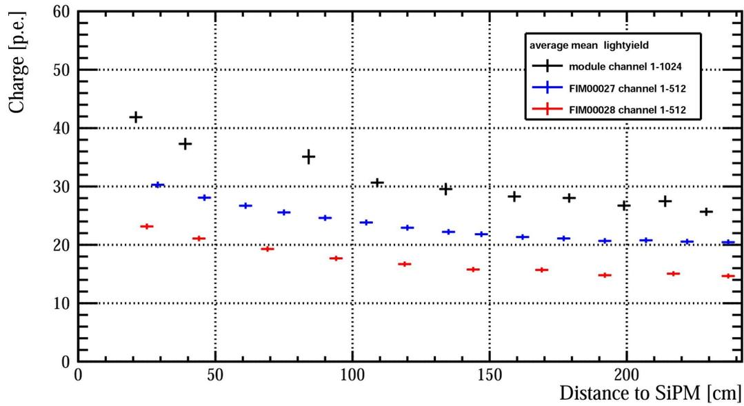
Figure 6.5: Measured attenuation over 10 different positions
