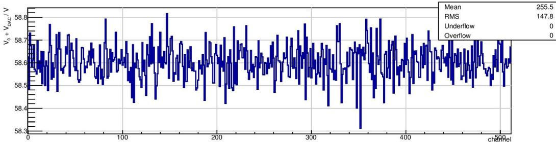
Figure 4.12: Measured breakdown voltages for every channel after gain calibration
