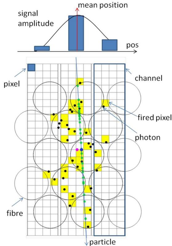
Figure 3.11: Schematic of a particle passing a fibre mat with five layers. The signal amplitude is proportional to the total number of firing pixel as one pixel can detect one produced photon. The fibres are not aligned to the channels.[1]
