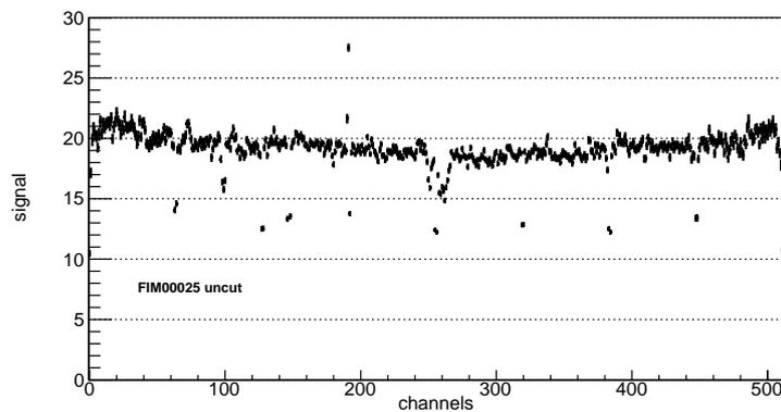
Figure 5.6: Light yield of the uncut mat FIM00025 with using the cluster algorithm
