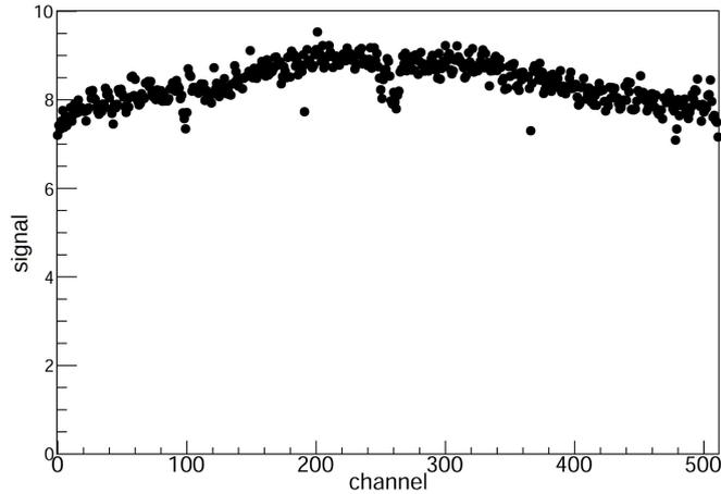
Figure 5.5: Light yield of the uncut mat FIM00025 without using the cluster algorithm
