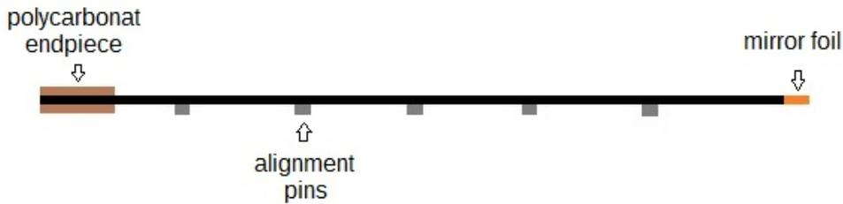
Figure 5.1: Schematic of a mat. The pins are used for alignment.
