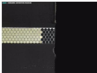
(b) Taken from the right side with the pins up. The fibres or the mirror at this edge is clearly damaged.
