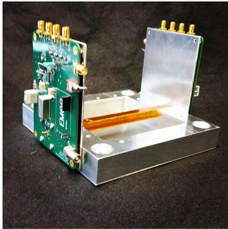
Figure 4.4: Trigger used for the setup to measure the light yield of the fibre mat. The bar which is covered in kapton tape is the scintillator. The green PCBs hold the read-out electronics
