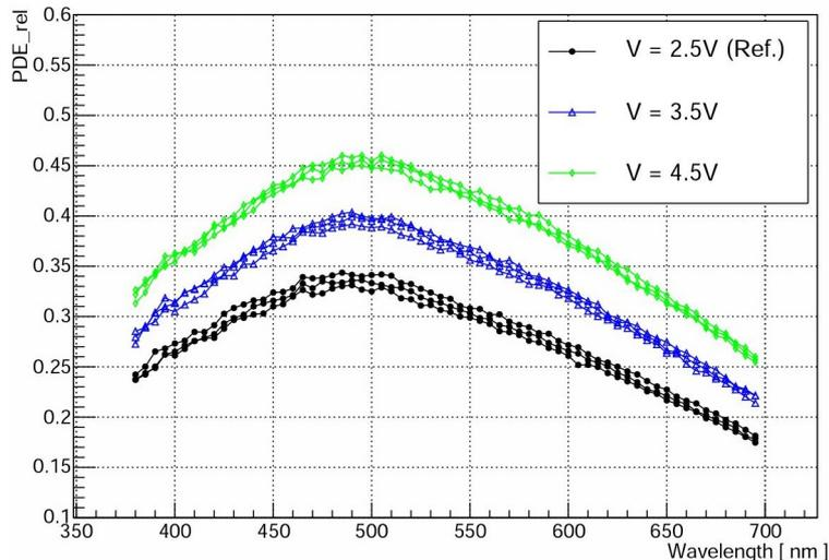
Figure 3.9: PDE for different over-voltages. The peak for  $U_{OV} = 3.5$  V is at the wavelength of 490nm with 39% [2]
