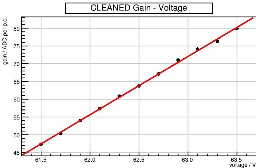
Figure 4.9: The Gain per ADC value is plotted against the operational voltage. With a fit the line can be extrapolated. The intersection point with the y-axis gives the breakdown voltage.
