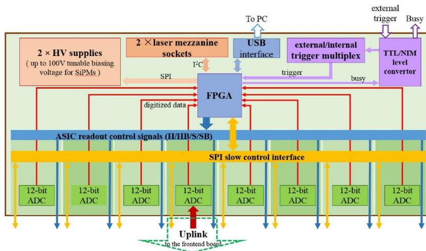
Figure 4.3: Buildup of the USB-Board [2]
