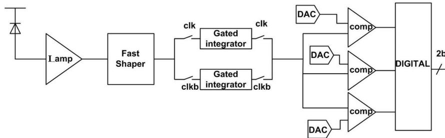
Figure 3.10: Schematic of the stages of the readout of one channel [1]
