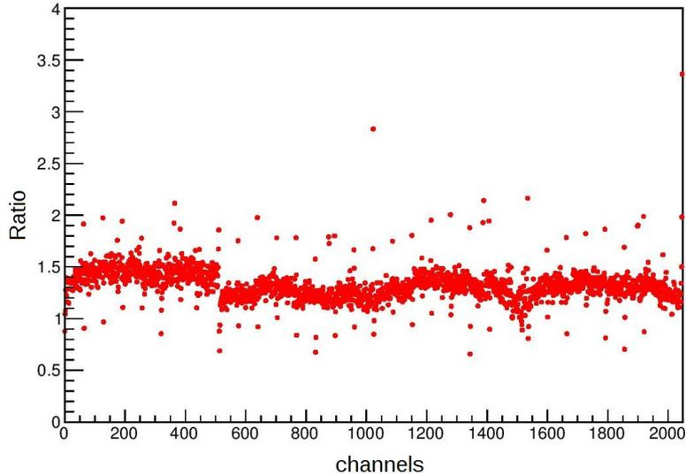
Figure 6.4: Ratio of the light yield of the module in comparison to the light yield measured from the single mats with beta-source
