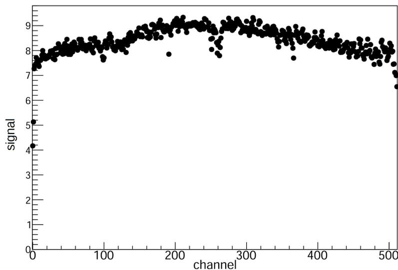
Figure 5.7: Light yield of the cut mat FIM00025 without using the cluster algorithm
