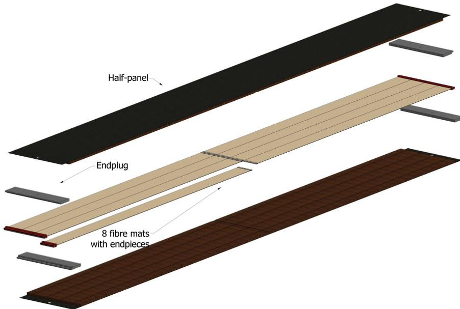
Figure 3.6: Exploded view of a module. The 8 fibre mats are placed with the mirror inside. The module is covered to guarantee light tightness [8].
