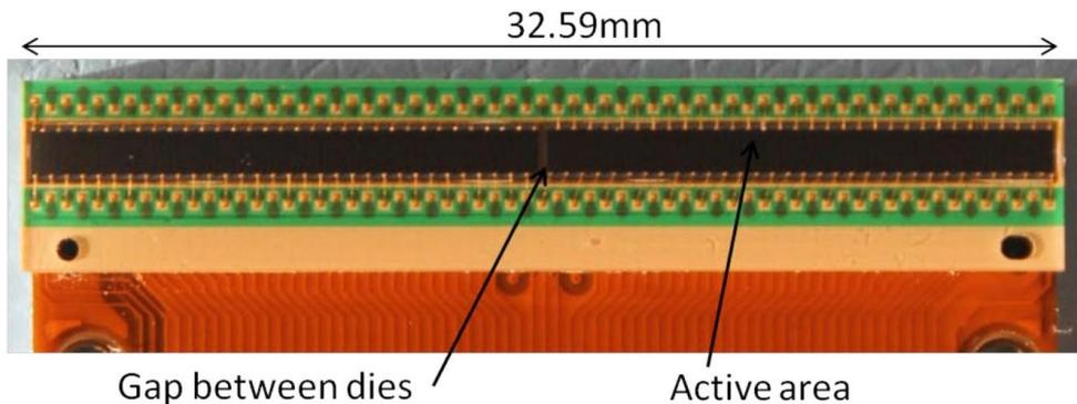
Figure 3.7: Overview of one SiPM array. The gap between the two dies can be seen [1].
