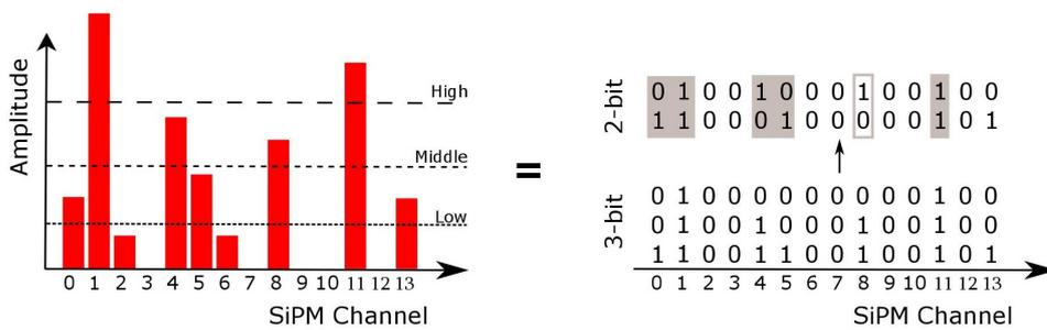
Figure 3.12: Left: Channel Clustering with three thresholds, right: 2-bit and 3-bit representation of it [2]
