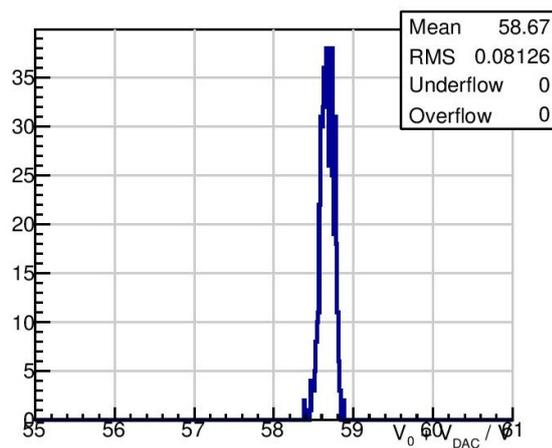
Figure 4.11: RMS for the breakdown voltage over all channels before gain calibration
