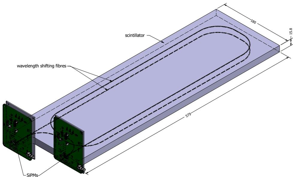
Figure 6.2: Schematic of the trigger used for the module measurements
