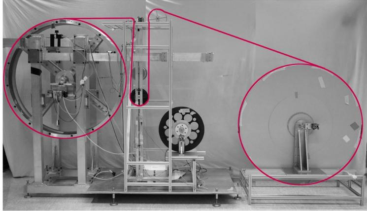
Figure 3.4: Prototype of the winding machine. On the right is the fibre spool, the winding wheel is on the left. The tension is controlled by a smaller weighted wheel that can be seen in the middle. [2]
