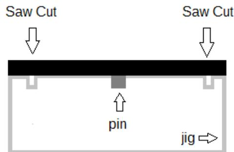
Figure 5.2: Schematic of the longitudinal cut set up. The pins are used for alignment. A saw cuts away the excess fibres.
