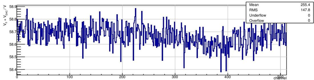
Figure 4.10: Measured breakdown voltages for every channel before gain calibration
