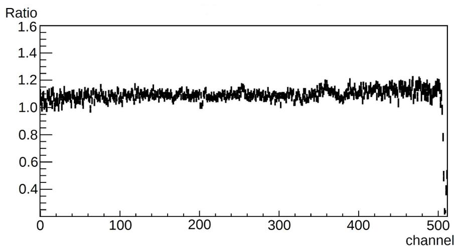
Figure 5.4: Ratio between the light yield of cut and uncut mat FIM00043
