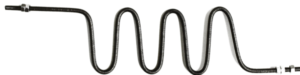
Figure G.9: Shunt resistor for the supermodule burn in test (Chap. 5.2). Bended V4A steel from Hornbach. High currents cause measurable voltage drops also over thick copper cables. This voltage drop has been used to efficiently check various connections in the low voltage cabling.
