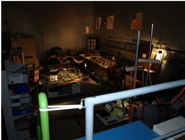
Figure G.4: The ALICE TRD as it was presented at opening days at CERN in April 2008. On the right side: Opened TRD multiwire proportional chamber. Center right: One out of 18 TRD supermodules partly equipped with chambers. Center Left: TRD chambers with mounted front end electronics (Readout boards equipped with MCMs) performing the gas leak test (see K). Left behind the cabin: Place and electronics for supermodule testing and the pretrigger development.
