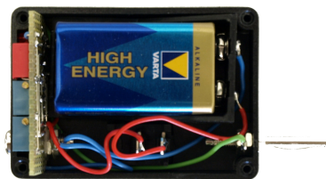
Figure G.8: Frequency generators. At one end of a cable a unique frequency is feed into each cable of the bunch. On the other side of the bunch the cables are identified via a frequency measurement with an multimeter between cable and ground.
