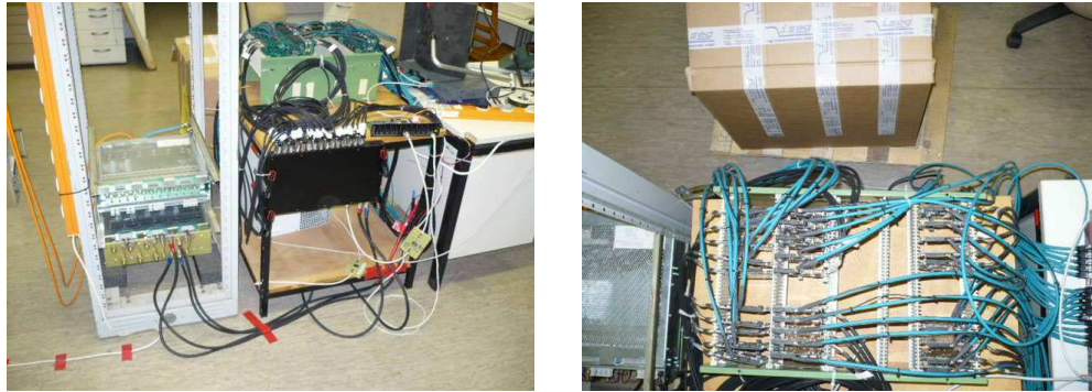
Figure 4.2: Pictures from the teststand in the lab in Heidelberg. The left picture shows an overall view of the teststand. In the crate on the left the backpanel of the power supply with the attached power distribution box and the power control unit is shown. The wooden table in the middle hosts the stand for the 30 DCS boards. A top view of the 30 DCS boards is shown in the right picture. In this picture the blue cables are the Ethernet cables attached to the Ethernet switches. The black cables are the power cables connected to the 30 output channels of the PDB.
