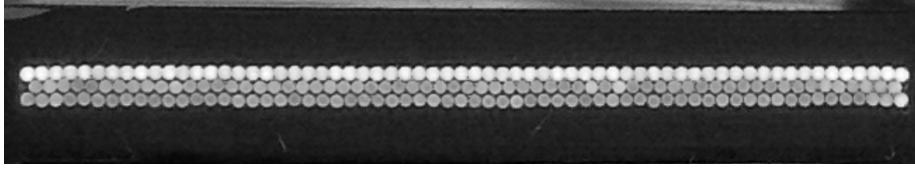
Figure 4.15: Cross section of a fibre ribbon [23]
