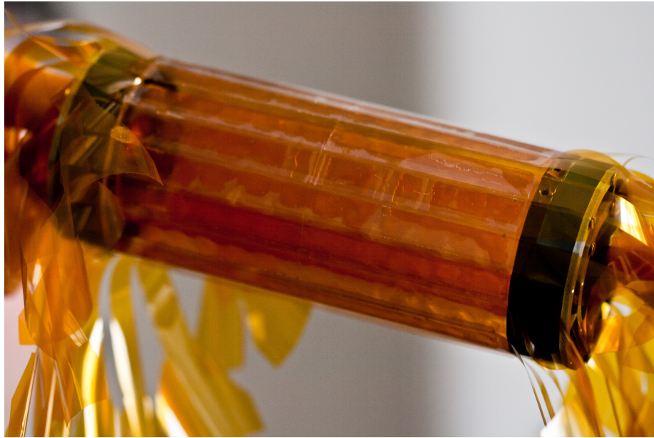
Figure 4.10: Prototype of the inner double layer of the pixel tracker
