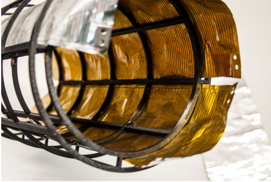
Figure 5.12: Photo of the 3D-printed support structure with three segments of layer 3 glued to it
