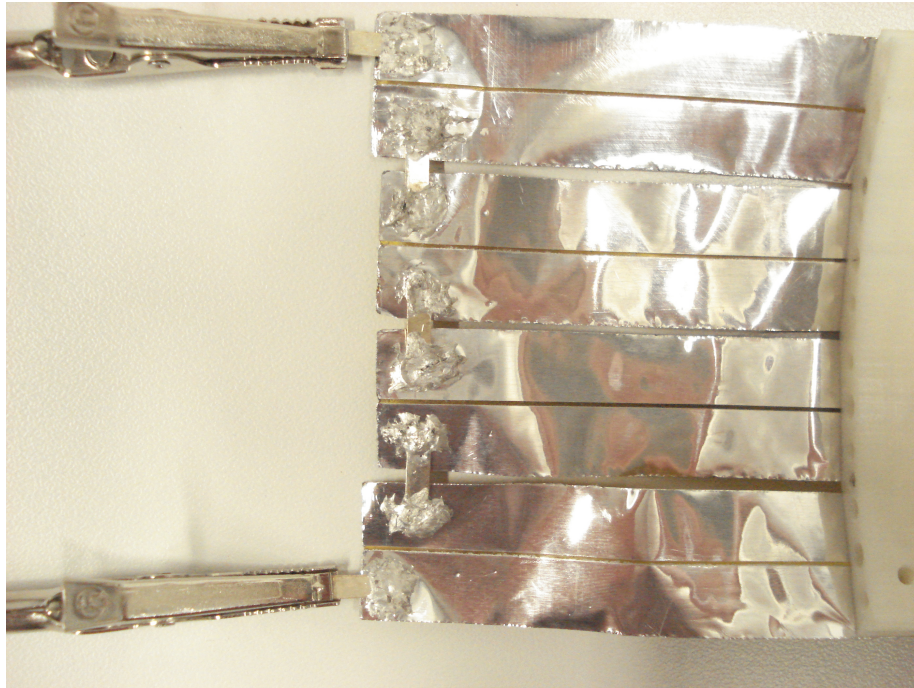
Figure 5.31: Electrical connections of the heating stripes of one module attached via ultrasonic soldering
