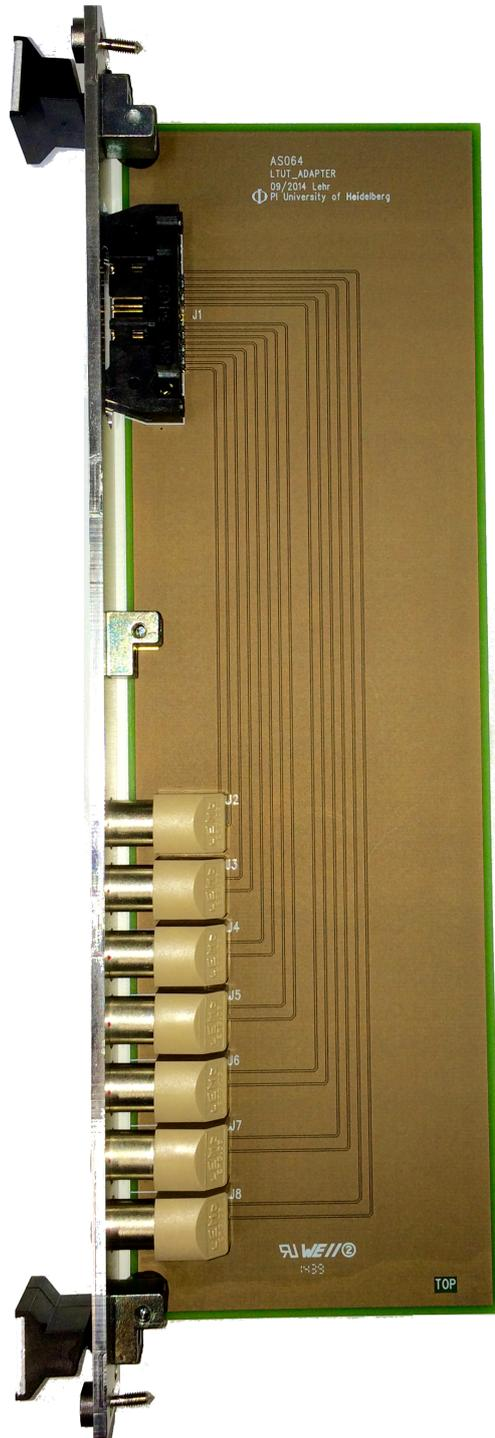
Figure D.3: Picture of the passive adapter between the LTU and the LTU-T.
