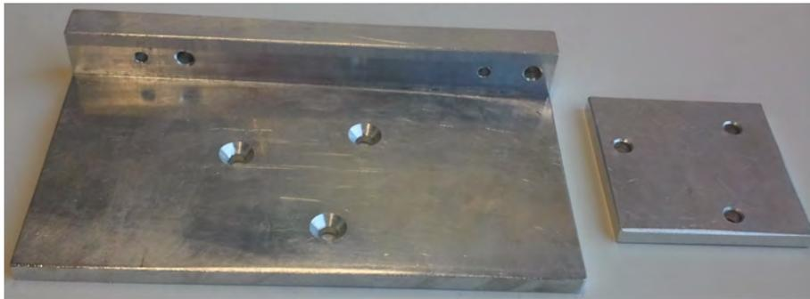
Figure E.1: Picture of the mechanical adapter to mount the MuPix PCBs on the rotation stage at the testbeam area T22 at DESY.
