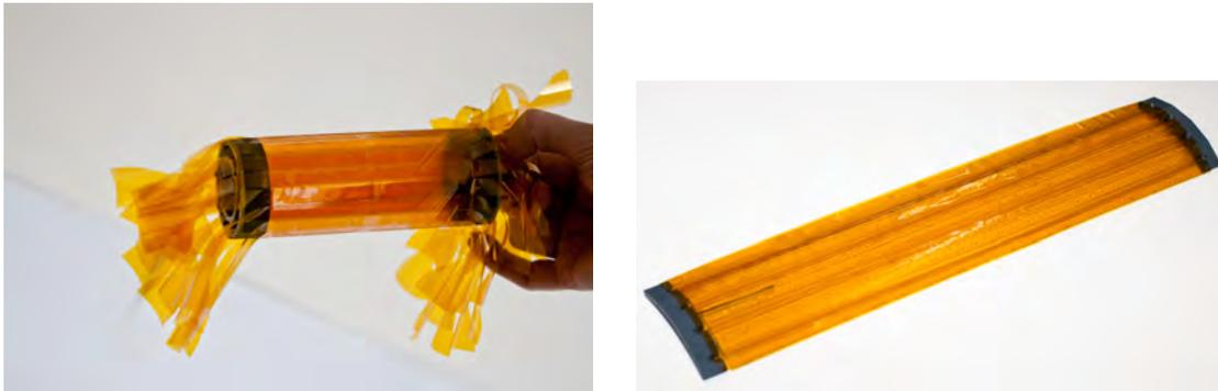
(a) Most inner pixel layer prototype of the detector (b) Prototype of a segment of an outer pixel layer
