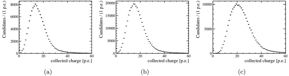
Figure 29.1: Light yield distributions of clusters found in the DUT of all accepted events for tracks at a distance of (a) 240 cm, (b) 120 cm and (c) 50 cm from the SiPM arrays. The angle between the surface vector of the module and the beam is  $0^\circ$ . The light yields are not corrected for crosstalk.
