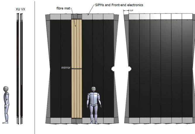
Figure 27.1: Sketch of the Scintillating Fibre tracker.
