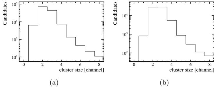
Figure C.3: Cluster size distributions of clusters found in the DUT of all accepted events when applying the foreseen LHCb thresholds of (1.5, 2.5, 4.0) for tracks at a distance of (a) 240 cm and (b) 50 cm from the SiPM arrays. The angle of the module with respect to the beam is  $10^\circ$ . The light yields are not corrected for crosstalk.
