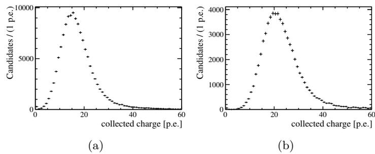
Figure C.1: Light yield distributions of clusters found in the DUT of all accepted events for tracks at a distance of (a) 240 cm and (b) 50 cm from the SiPM arrays. The angle of the module with respect to the beam is  $10^\circ$ . The light yields are not corrected for crosstalk.
