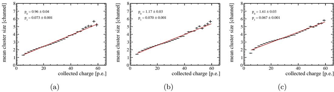
Figure 29.3: Mean cluster size as a function of the collected charge for tracks at a distance of 240 cm to the SiPM arrays and an angle of the module of (a)  $0^\circ$ , (b)  $10^\circ$ , and (c)  $20^\circ$ . The fit function is a straight line with offset  $p_0$  and slope  $p_1$ .
