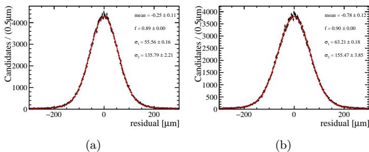
Figure C.5: Residual distributions of the SciFi cluster positions with respect to the reconstructed TimePix tracks using the (a) charge-weighted mean and (b) PACIFIC-like hit-weighted mean for tracks at a distance of 120 cm from the SiPM arrays. The angle of the module with respect to the beam is  $0^\circ$ .
