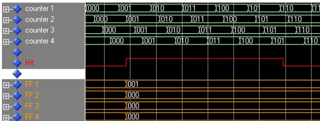
**Figure 5.6:** Working principle of the fast counter method. To reach a time bin size below the counter period, four counters are used. The counters are running with the same clock frequency and are phase-shifted by  $90^\circ$  with respect to each other. The rising hit signal (red) triggers the latching of the four counter values (green) into the flip-flops (orange). The absolute time of the hit signal can be calculated from these four values.
