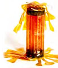
(b) Prototype of inner layers. The silicon pixel sensors are replaced by glass.
