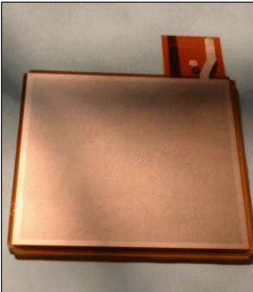
GEM foil glued to frame, complete CASCADE module
