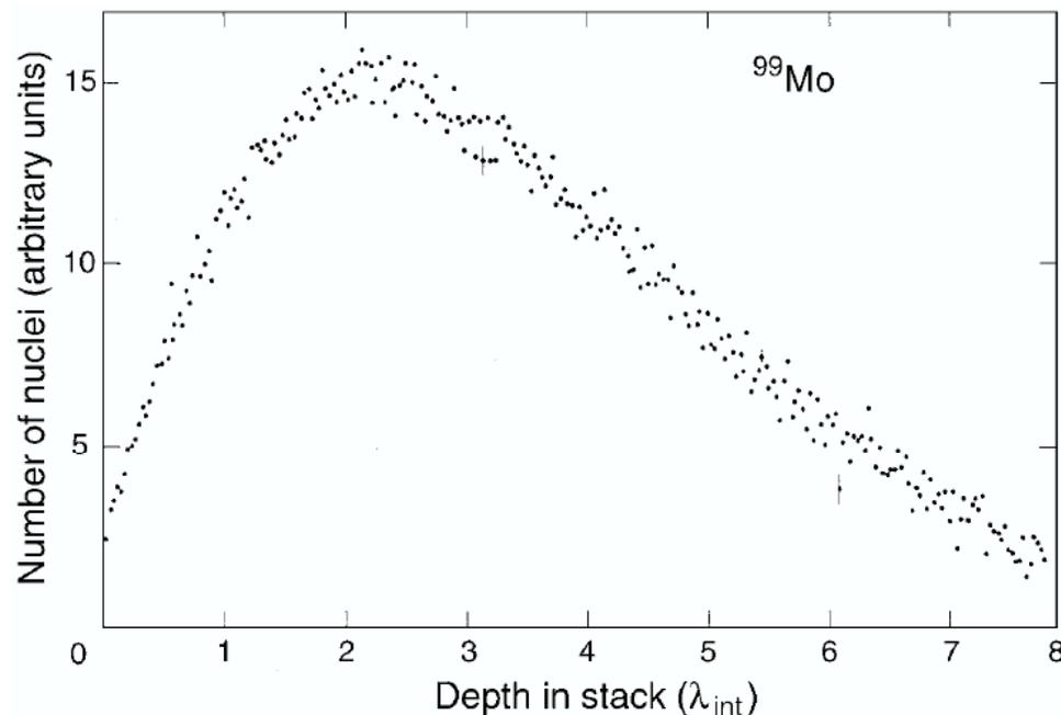
long. shower profile for 300 GeV  $\pi^-$  into block of U; measure radioactivity of a fission fragment
