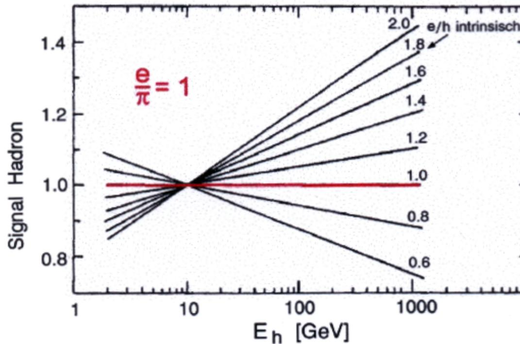
hadron signal in different sampling calorimeters
