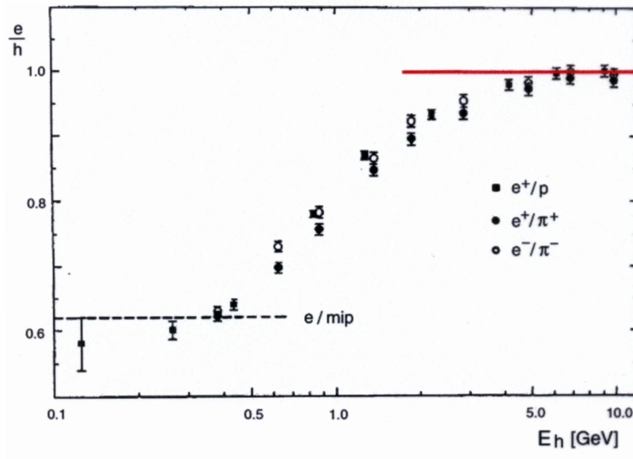
measured ratio of electron/pion signals at (ZEUS) for  $E \geq 3$  GeV nearly compensated
