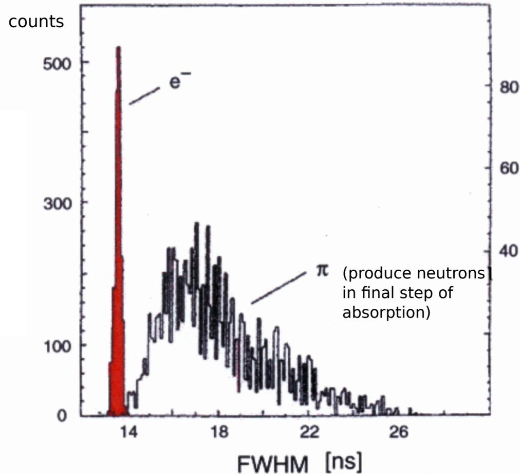
size of signal depends on integration time – variation in integration time of electronics can enhance hadronic signal (used in ZEUS calorimeter)
